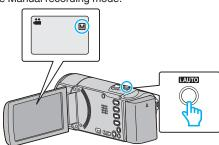
• If the mode is **i.A.** Intelligent Auto, press the i.AUTO button to switch to M Manual.
